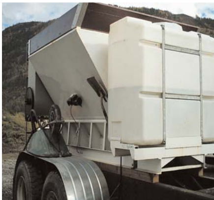
Large Capacity Water Tank for mixing and clean out.
